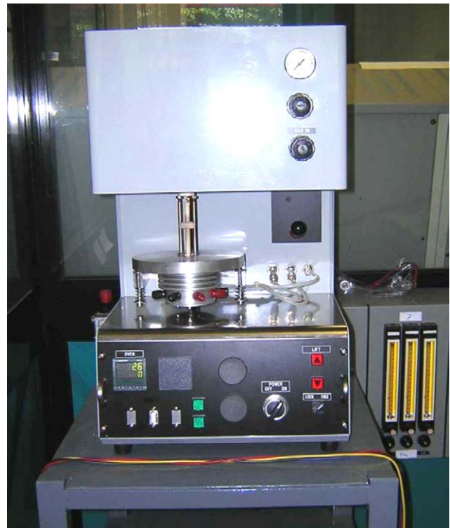
Fig. 4. Cell for the measurement of electrical conductivity.
